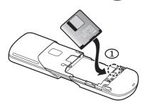
Press the battery down into the battery slot (2).
