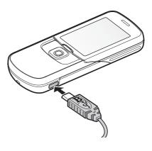
The charging time depends on the charger used. Charging a BP-5M battery with the AC-6 charger takes approximately 2 hours and 15 minutes while the phone is in the standby mode.
