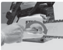
Tensioner screw on a Stihl chainsaw
