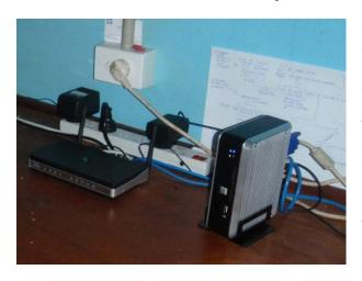
On the left is an example of a low cost, low power fanless PC computer costing less than USD 800, which consumes only 10-15W of power. Ideally, two network adapters (NICs) should be used, one which can connected to the Internet (optional) and one with the local network (LAN) with the wireless access point(s). Depending on local sunshine/insolaltion, one 130W solar panel may be sufficient to support this device 24 hours per day.
