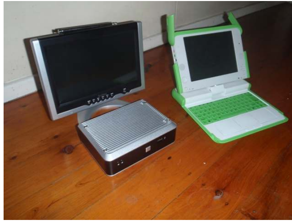
An example of a small, low power, “eBox” suitable for a solar-power
