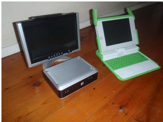
An example of a small, low power, “eBox” suitable for a solar-power Cost is about USD 500 or less. Power consumption (with screen off) is less than 15W Storage is 160-300GB.
