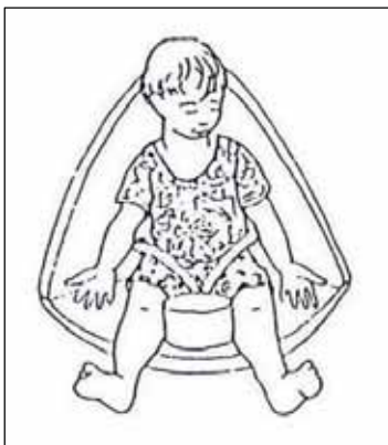
Fig. 20.33: A CP chair or corner seat can be made from wood, foam or cardboard
